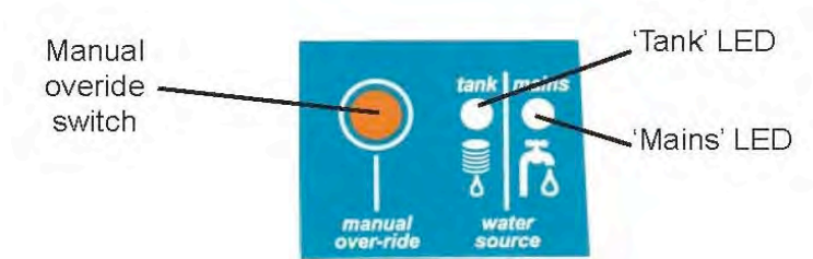
Figure 8: Onga WaterSwitch Tank / Mains Water Indicator LED Lights (Located at back of WaterSwitch)
